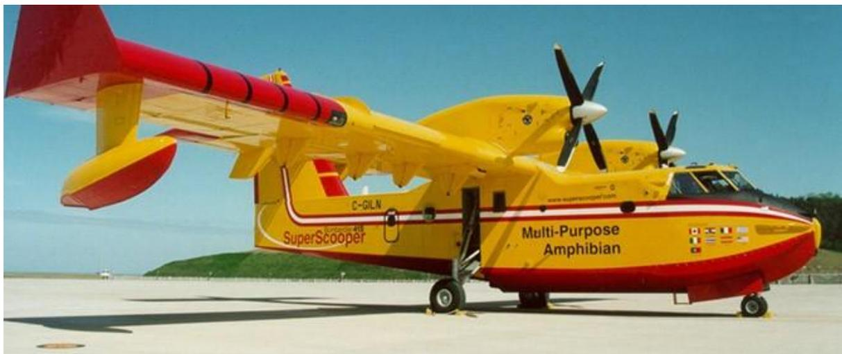
Figure 5: Bombardier 415 MP - Combining a state-of-the-art surveillance suite with direct water intervention capabilities.
