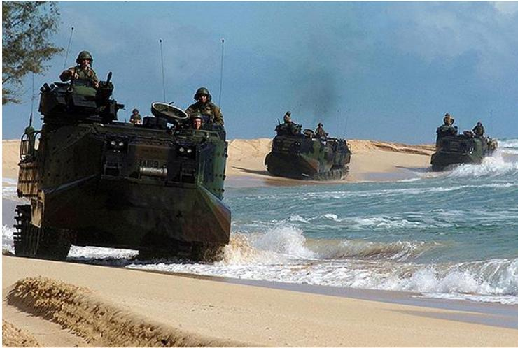
Figure 6: AAV7A1 Assault Amphibious Vehicle<sup>8</sup>
